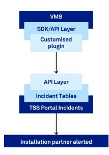
Customised alarms are pushed from the Video Management system to the customised alert plugin, into the API layer which loads the data into the relevant table, generating the required incident and alerting the relevant installation partner.
