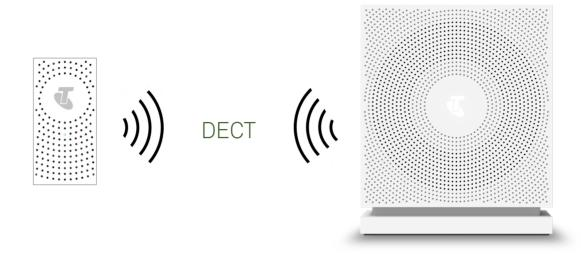
The Telstra Voice Extender (TVE) connects wirelessly via DECT to the DECT base inside your Telstra modem. The RJ11 telephone port located at the base of the TVE then provides a standard telephone wall socket in your house allowing you to connect any standard cordless or corded telephone wirelessly between the TVE and modem.
