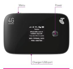
Press the Menu Button to scroll through the Menu and use the Power Button to select. From the Menu you can view device info including Wi Fi Name and Password, view Wi Fi Bands, enter Wi Fi Protected Setup (WPS) and update device software.
